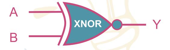
A XNOR gate is true Input A AND Input B are both true or both false.
