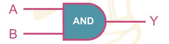
With most logic gates, we will have more than one input, causing our truth tables to be bigger. For two inputs, our truth table will have **four** possible outcomes.
