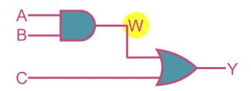
The "stepping stone" W is the output for the individual AND gate. The "stepping stone" W is also an input for the individual OR gate.
