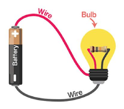
For current electricity to flow, it requires a circuit: a closed, never-ending loop of conductive material
