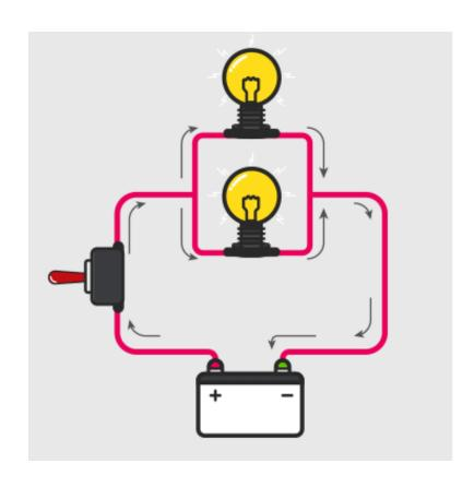
Parallel circuits have two or more components connected in such a way that each component is connected *directly to the source*. If one component is removed current will continue to flow to the other components in the circuit and will continue to work.
