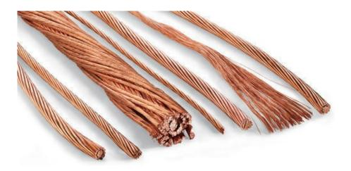
Stranded wire is made of a bundle of numerous solid wires bound together.
