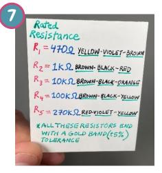
Write the rated resistance values for each of the resistors on the back of the card.
