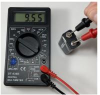
Touch the red probe to the positive (+) terminal of the battery and the black probe to the negative (-) terminal of the battery.
