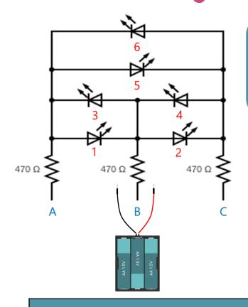
Once you have built the circuit and tried to light up LEDs #1, 2, 3, 4, 5, and 6 use the data table to indicate what points (A,B, or C) the positive (red) and negative (black) leads from the battery were connected to.
