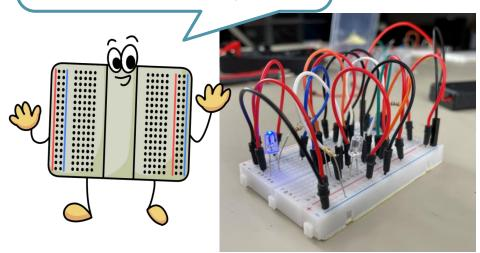
Solid core wires lay flat and can make it easier to see the connections in a circuit when there are many connections. Short wires can be used to connect components located near one another. Jumper wires allow any two points in a circuit to be easily connected. But when there are many connections in a circuit it can sometimes be difficult to see through the tangle of wires to troubleshoot a circuit.
