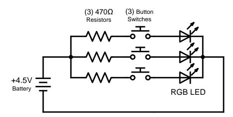
RGB LEDs can have power (+) attached to multiple anode pins (red, green, blue) at the same time.
