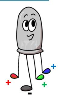
The RGB LEDs provided in the kit are called common cathode (-) LEDs.
