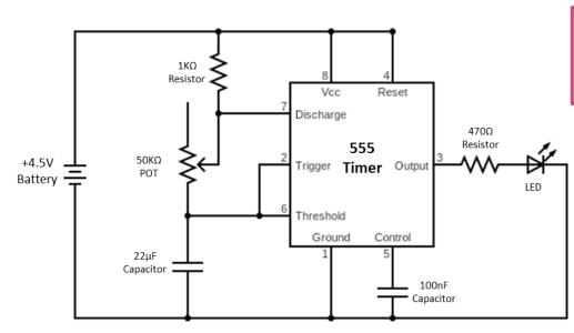
The notch on the chip identifies the top of the chip to help you find pin 1.
