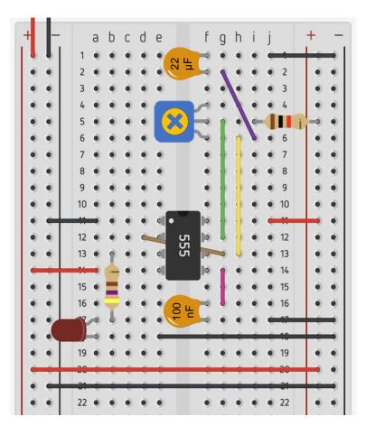
The pins are numerically arranged counterclockwise from the top left pin.
