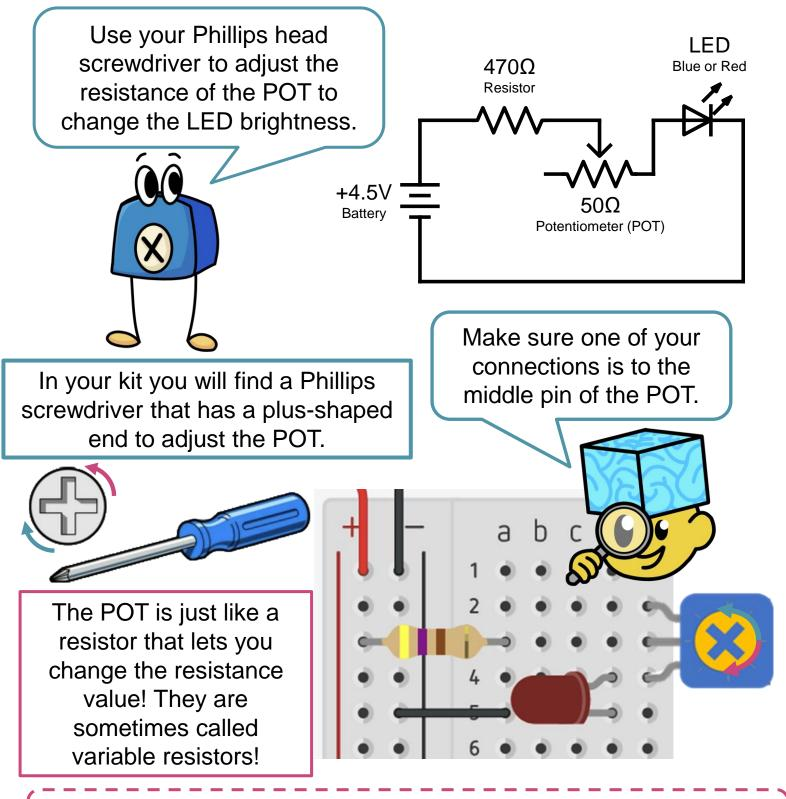
Turning the POT one direction will brighten LED. The other direction will dim the LED. The direction will depend on how you put the POT into the circuit.
