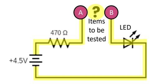
Turn on the battery pack and connect the testing wires to the various items you will be testing to determine which ones conduct and which ones do not!
